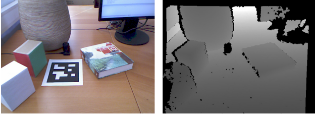
Figure 9: The left image shows the RGB color input stream and the right image shows the depth values of the Microsoft Kinect sensor.
